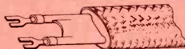
Fig. 5 Replace the twin-lead from the antenna terminals on the back of the cabinet to the tuner with shielded 300-ohm cable to minimize the pickup of leading ghosts. This is an alternate to Figure 4, in case the customer still wants to be able to use an external antenna.
